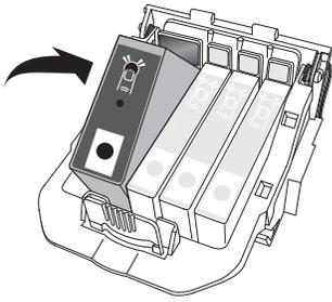
7. Place the ink cartridge into its corresponding colored slot.
