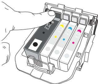
3. Press the colored tab on the back of the print head that corresponds to the used ink cartridge. The ink cartridge pops up slightly.
