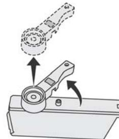
6. Remove the ink protective cap from the ink cartridge.
