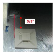
4. Install a second cable tie mount to the right of the cable tie mount from the previous step. It should be located one inch below the bracket, which is approximately even with the middle of the cable tie mount installed in the previous step as shown in the image below.
