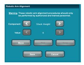
3. Press the Move button and the robotic arm will perform the calibration process.
