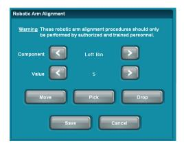
**NOTE:** Components (except for the Special Components) have calibration values between -32 and 32 that adjust the position of the robotic arm. Left bin and right bin calibration values are limited to -20 through +20 for the 84-series and 101-series recorders only.
