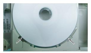
If the optical disc position in the optical drive tray is too far in or out, the optical drive position will need to be adjusted. If no adjustment is required, proceed to step 15.
