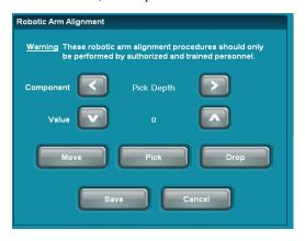
Press the Pick button. Watch the robotic arm body and note how much it is lifting up on the top guide rail. The optimal setting is to apply enough force to lift the weight of the robotic arm assembly, but not enough to push against the top guide rail. Hearing the stepper motor get overloaded can also indicate too much force. Too much force can also increase the chance of two discs being picked.
