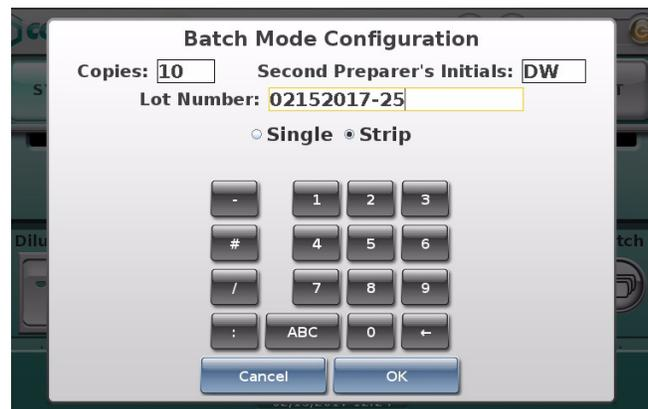
**NOTE:** In Batch Mode, up to 999 copies can be printed in one batch job. Up to 18 alphanumeric characters can be used for a lot number.
