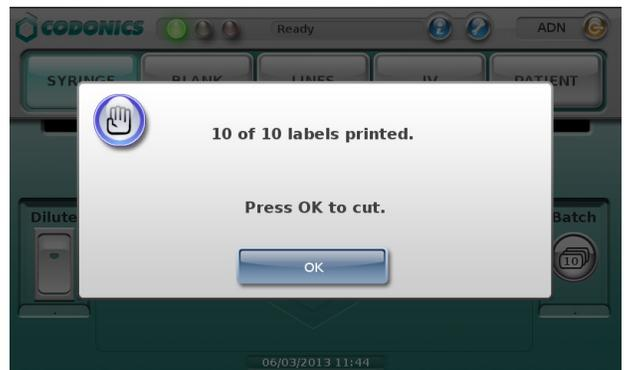
**WARNING:** Do not pull the strip of labels or try to tear the strip of labels. This can cause jamming and/or damage to the SLS PCS.
