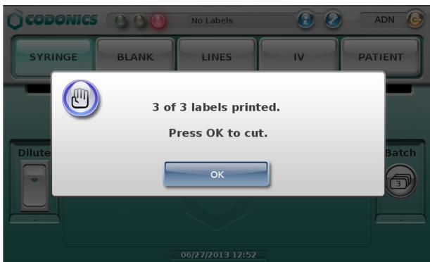
If the job is not complete, a dialog screen will indicate how many labels have printed, and will ask you to cut the labels and to load media.
