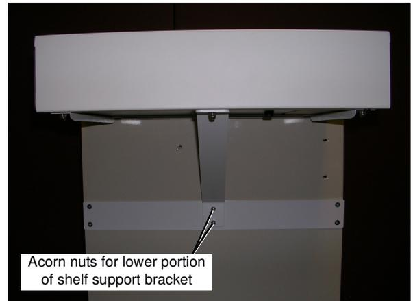
21. Tighten the four shelf support bracket acorn nuts using a 5/16-in. nut driver. Then tighten all four flat-head screws using a P3 Phillips head screwdriver to secure the lower support bracket to the side of the cart.
