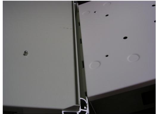
11. Make sure that the shelf is level front-to-back. If the shelf is not level, loosen the shelf rail mounting screws and adjust it as necessary.
