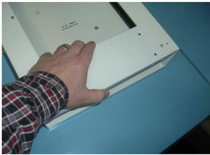
5. Install the power supply bay into the opposite side of the shelf frame. Secure it to the shelf frame with the four pan-head screws that you removed in step 3.
