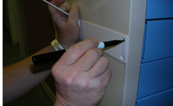
NOTE: If the Blue Bell top shelf support rail is installed use a 6-inch level aligned with the holes of the lower support bracket to determine the location of the mounting holes. Mark the locations on the cart with a permanent marker.
