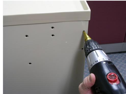
**NOTE:** A step drill bit is recommended for maintaining the best hole location and quality.
