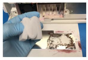
12. Press the new ink filter into the ribs as shown.
