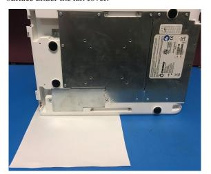
5. Use a T10 screwdriver to remove the two screws securing the fan cover. Save the screws for step 14.
