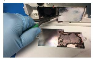
The ink filter will be saturated with ink making it messy to handle. Use a pair of needle nose pliers to remove the filter and discard it.
