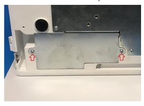
Carefully remove the fan cover and lay it on top of the rag.
