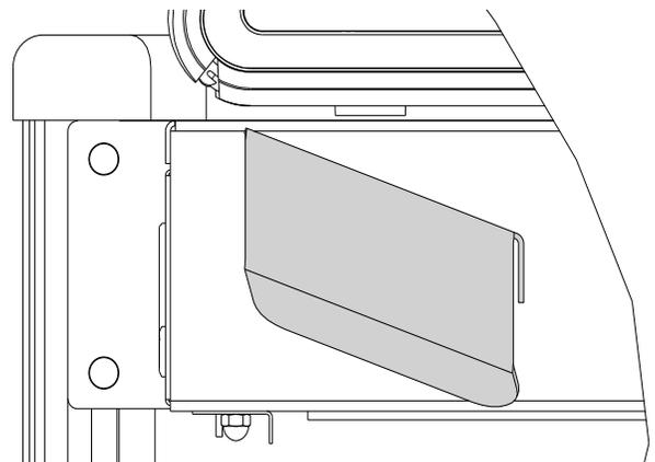
3. Press the holster onto the 500i shelf and apply pressure for 30 seconds to one full minute.
