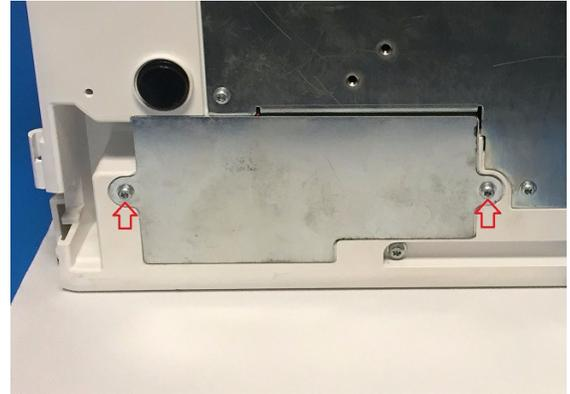
6. Carefully remove the fan cover and lay it on top of the rag.
