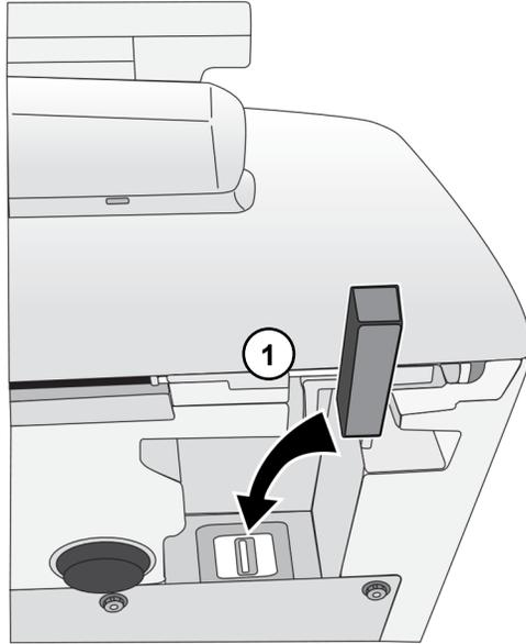
1. Insert the Wi-Fi adapter into the USB port at the bottom front right corner of SLS PCS.
