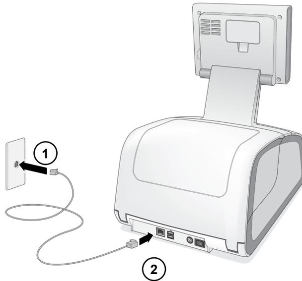
1. Connect the Ethernet cable to a hub or outlet that is connected to the network.
