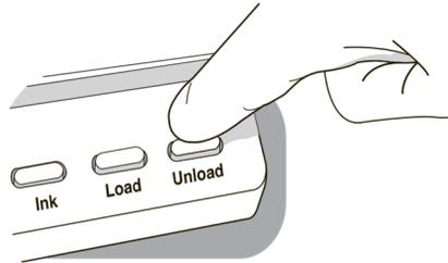
8. Press the Unload button to reverse any portion of the label media that is still in the media path.
