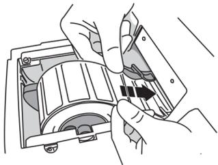
5. Place the label media below the media guides and into the feeder slot.
