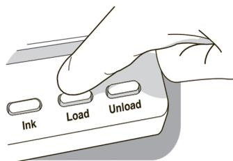
If required, press the Load button to advance the label media.
