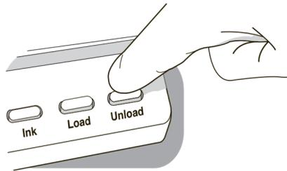
6. Press the Unload button to reverse any portion of the label media that is still in the media path.
