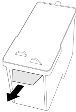
5. Remove the tape that covers the ink cartridge print head.
