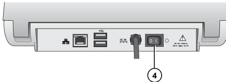
4. When shutdown is complete, turn off the Power switch.
