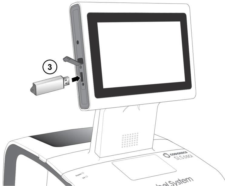
3. Insert the USB flash drive on which the update package or software is installed.
