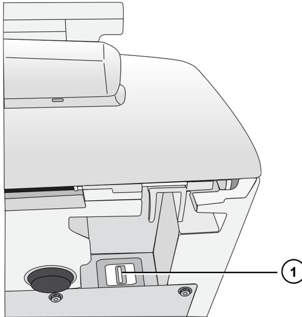
1. USB port for Wi-Fi adapter (bottom front right corner of SLS PCS)
