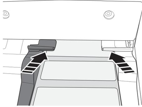
6. Feed the label media until SLS PCS automatically feeds it through the media path. You might need to hold the label media in place for a few seconds.
