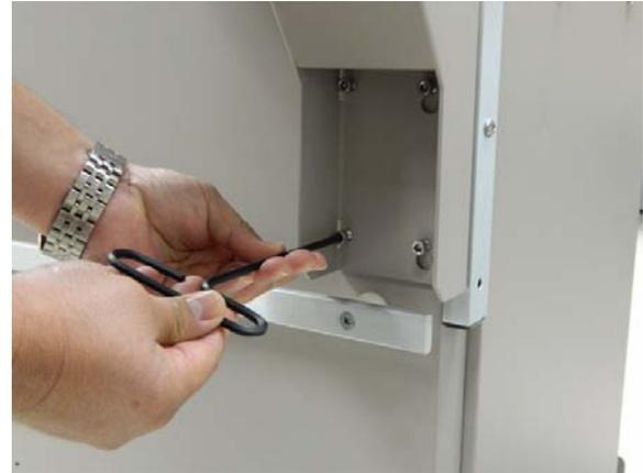
7. Grasp the accessory arm mount and make sure that it is attached securely to the Pyxis Anesthesia system 3500 unit.
