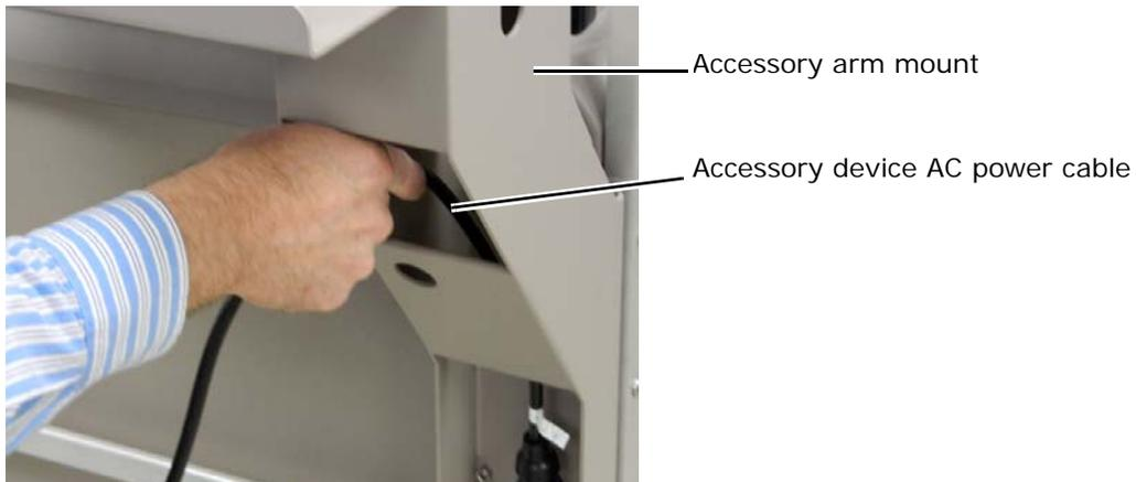
12. Insert the accessory device AC power supply into the accessory arm mount.
